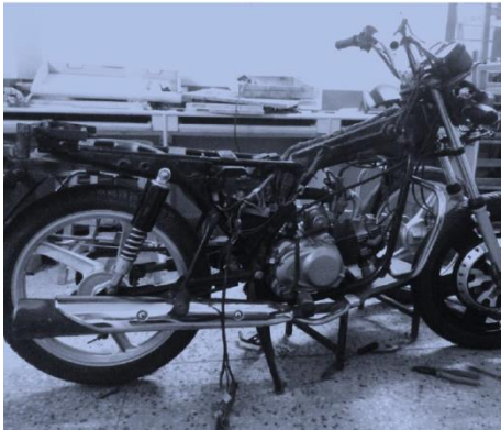
Hybrid Electric Motorcycle (IC Engine + Hub mounted Motor at front wheel)
