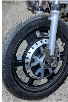
Hybrid Electric Motorcycle (IC Engine + Hub mounted Motor at front wheel)
