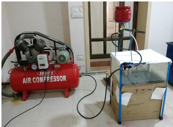
Abrasive Jet Machine with demonstration of machining on MS plate and Glass
