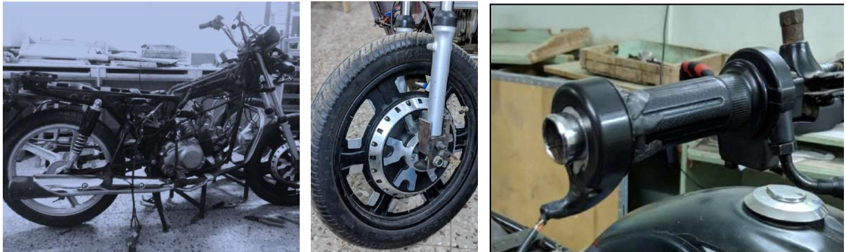
Hybrid Electric Motorcycle (IC Engine + Hub mounted Motor at front wheel)
